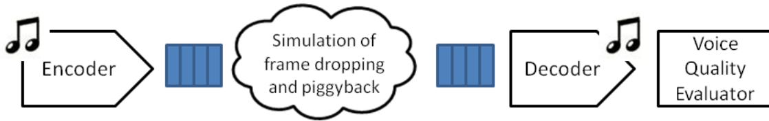
Fig. 6. The information flow of our methodology for computing audio quality under given network conditions.
